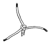
With the marlinspike or nail, lift one of the strands of the rope immediately below the Crown Knot and pass the end of one of the strands underneath it. Pull tight.
